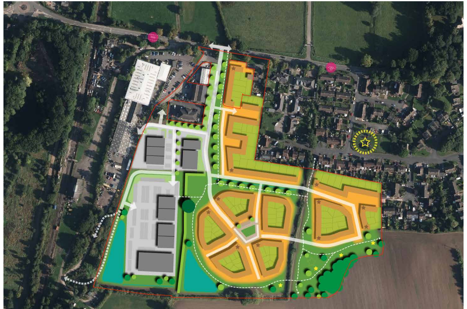
FIGURE 7 - DEVELOPMENT FRAMEWORK OPTION A: The above figure shows a Development Framework for the site's development on the basis of Access Option A. That option would involve provision of a central access road close to the eastern site boundary, and therefore the retention of the existing employment premises to its west, which would in turn tie in with additional employment provision at the site's western corridor. As the new access route enters the site at its north, land to the east could be developed for residential use and would wrap the adjacent residential edges; providing sufficient separation distances to sensitively respond to their amenity. Residential development would also be focused at the site's centre and south-east, and should be supplemented by generous areas of public open space and landscaping. A landscaped open space corridor through the centre of the site would provide a buffer between employment and residential uses, and should also incorporate drainage features.
