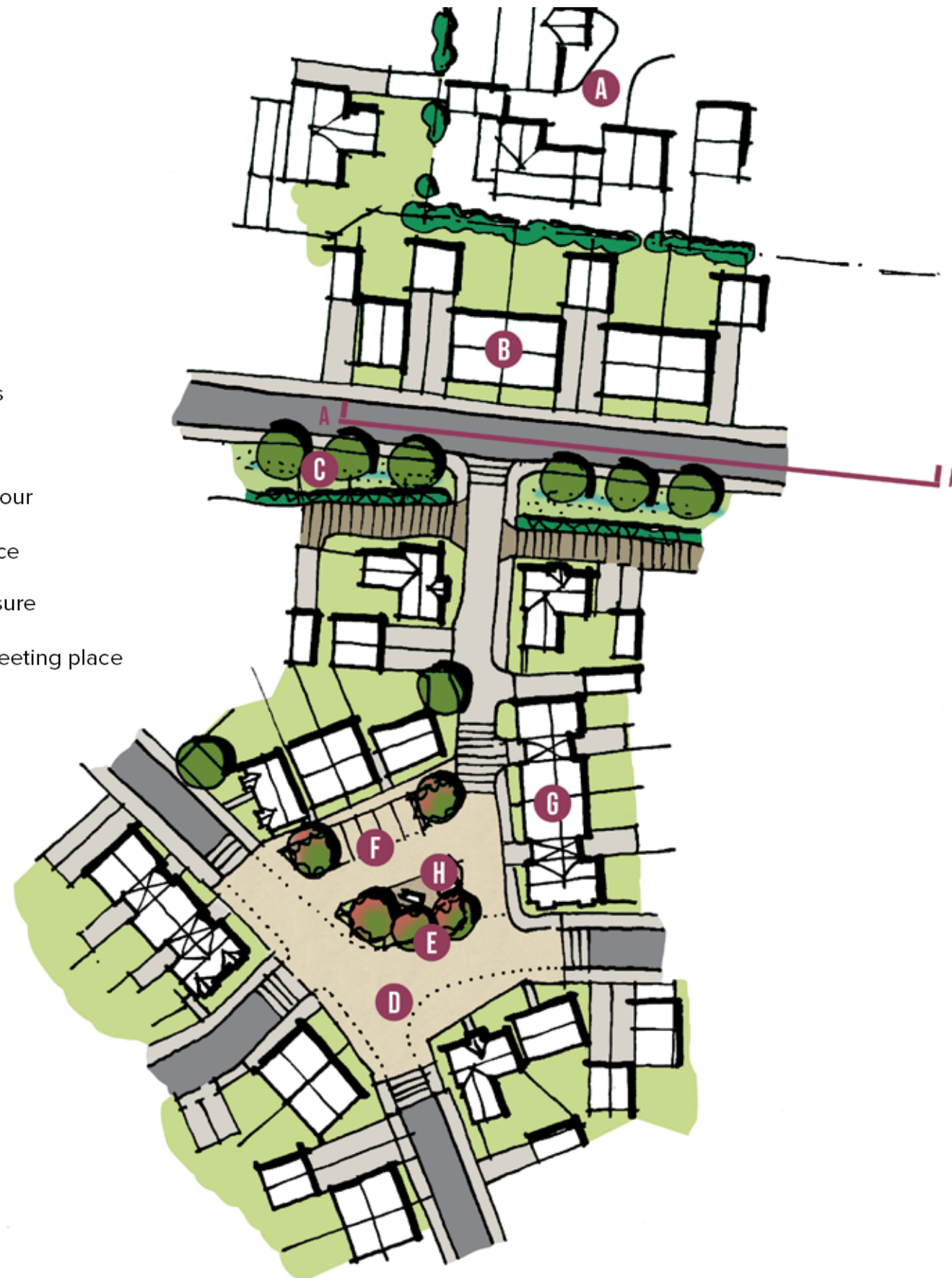
FIGURE 11 - SKETCH 2, RESIDENTIAL SQUARE @ 1:750: Shows how the development proposals would sensitively respond to neighbouring bungalows to the north by limiting development at the north-eastern boundary to single-storey bungalows. The sketch also demonstrates how residential development should be provided as part of a 'residential square' that incorporates shared surfaces and focal spaces, seasonal planting and communal seating, and could promote a strong sense of enclosure.
